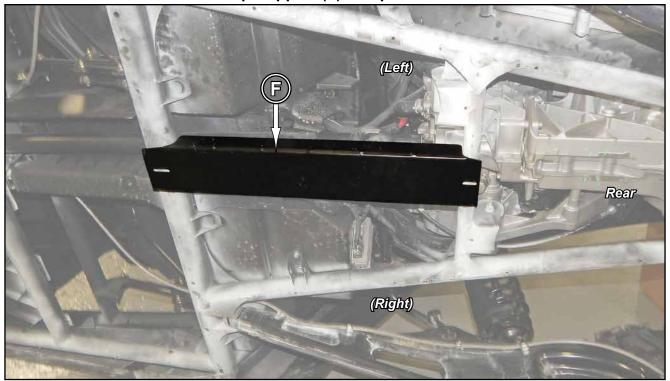
Install Rear Plate (E) with hardware shown.
