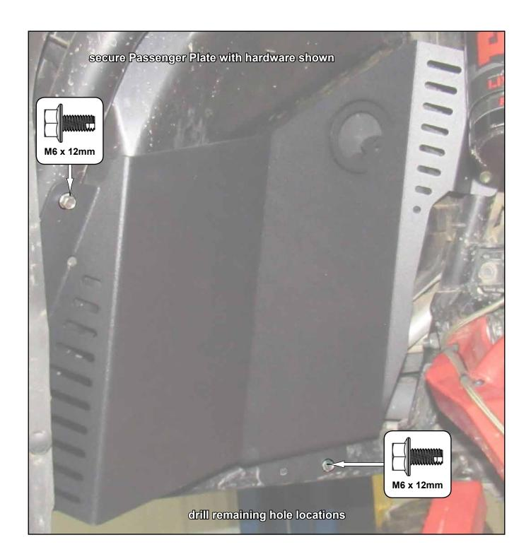
secure Passenger Plate with hardware shown; tighten completely
