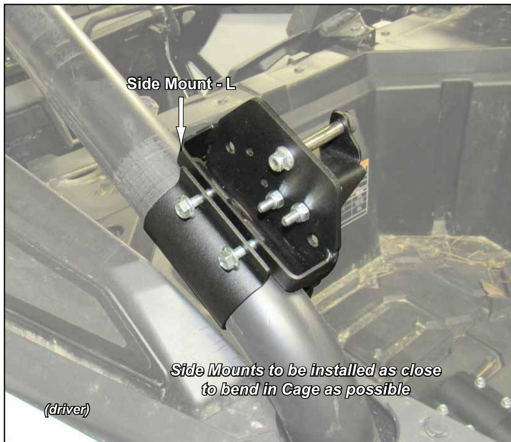
*Side Mounts to be installed as close to bend in Cage as possible*
