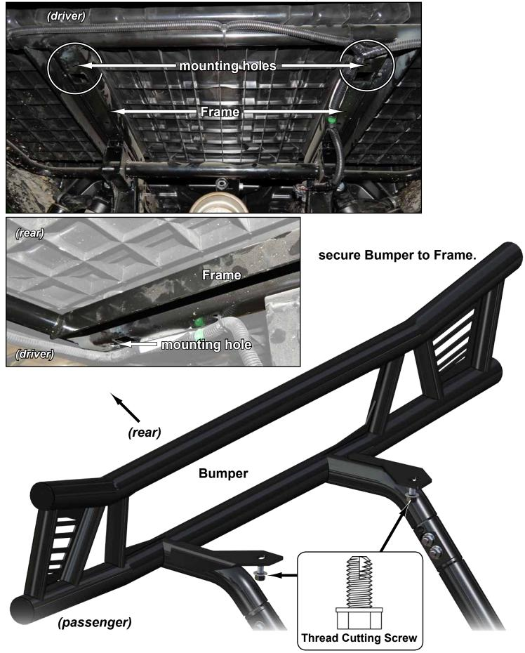
Align to machine and tighten hardware completely.
