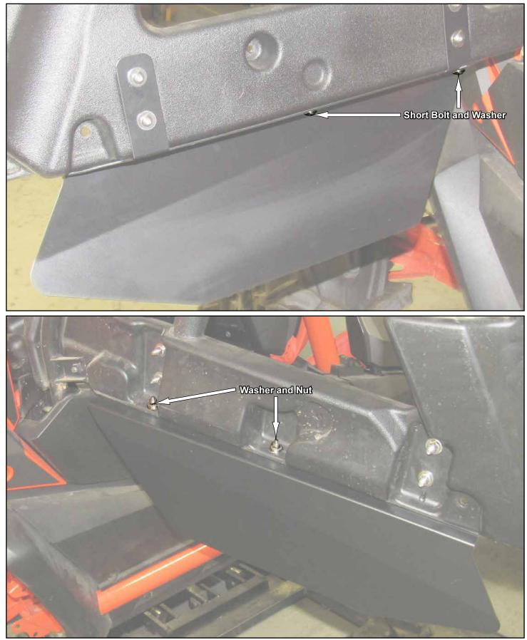
Reinstall stock Insert, tighten hardware completely, and repeat steps for Left Door. IN-DOOR-H-TALX4
