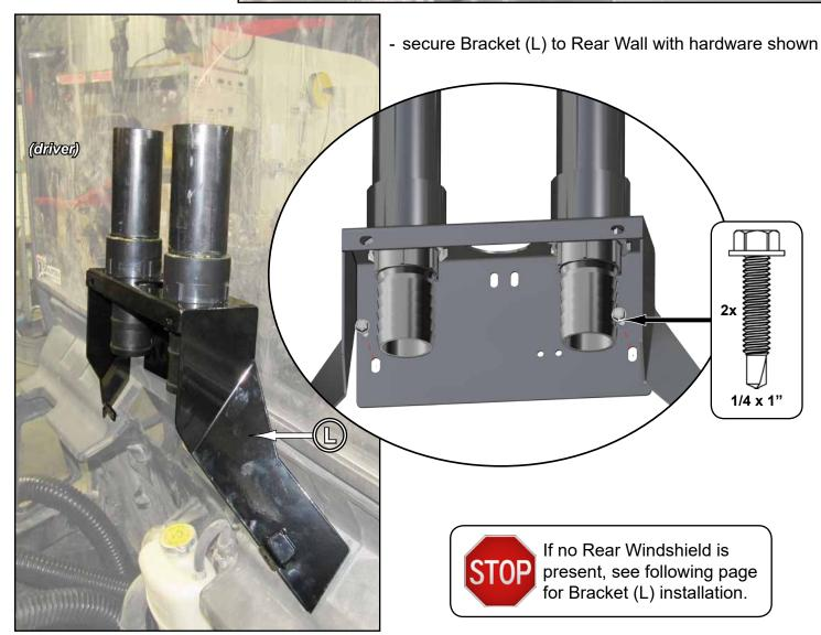
Spacers must be installed between Bracket (L) and Rear Wall if no Rear Windshield is present.
