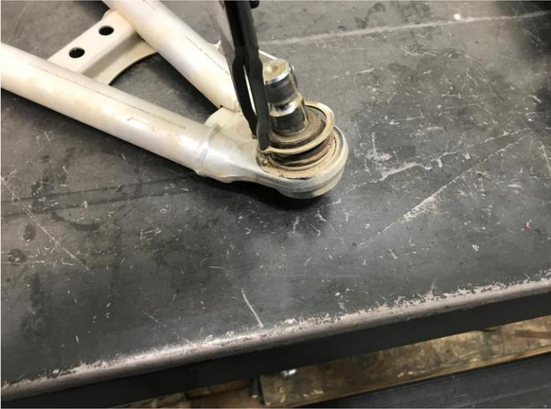
6. Using a press or vice use large sockets or tubing and press the ball joint out of the factory control arm.
