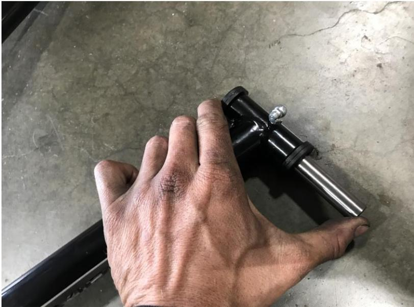
11. Place the arms in to the frame and install the factory hardware.
