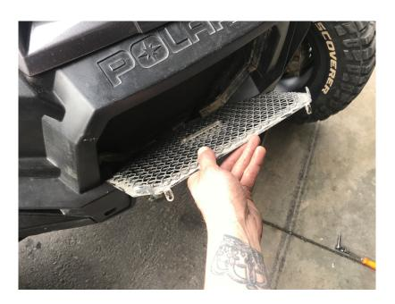
2. Place the bumper into its location and loosely install the two upper bolts into their mounting holes. Do not tighten at this time.
