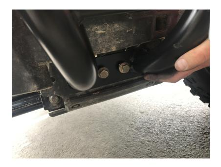
$4.\,\mathrm{Tighten}$  the two upper M10 bolts making sure the bumper is level.
