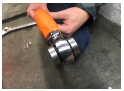
6. Place the small spacers and O-rings in the other end of the upper arm install it into the spindle. Make sure you go underneath the brake line.
