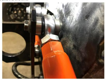
8. Measure the factory lower arm length, hole to hole. Adjust the joints in the high clearance arms to match. Install the lower arm into the spindle with the small spacers and O-rings.
