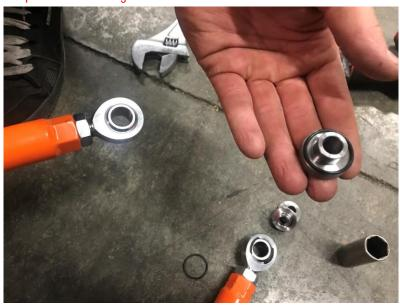
5. Spin the spacer in the joint lightly to get the O-ring to center itself. The only purpose of the O-rings is to eliminate "rattle" from the joints when the arms articulate.
