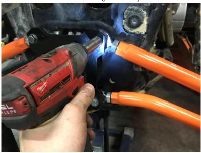
11. On the lower control arms with jam nuts loose. lightly rotate the arm away from the machine. This is to rotate the inner joint back to offset the front to back rotation. Now tighten the jam nuts. If this is not done the lower arm may contact the back of the frame.
