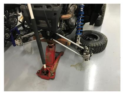
2. Begin to remove the factory upper radius arm by removing the 15mm or 18mm bolts. We recommend only doing one side at a time.
