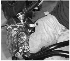
23. When you have reattached both upper and lower arms to the knuckle attach the entire assembly to the frame.
