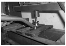
12. Install the factory ball joints into the new arms.
