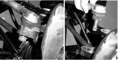
6. Because it is difficult to disconnect the upper and lower control arms from the knuckle assembly, it will be easier to disconnect them from the frame and pull the upper and lower arms off as a complete unit still attached to the knuckle. Once you have the assembly off you will have easier access to the cotter pin and castle nut that connects the arms to the knuckle.
