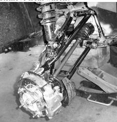
**3.** Disconnect the brake lines from the control arms. Disconnect the calipers from the hub/rotor assembly. **Do not disconnect then brake lines from the calipers!**
