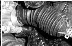
19. Next pull the boot back to expose the inner tie rod joint.
