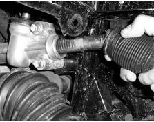
20. Place the steering stop clip between the inner tie rod joint and the rack and pinion. It is a tight fit, so you may have to force it on this is to ensure that the spacer stays in place.
