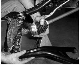
NOTE: Make sure to insert the axle into the knuckle when sliding the upper and lower arms into place on the frame.
