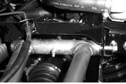
25. Connect the shock to the upper control arm using the factory hardware.
