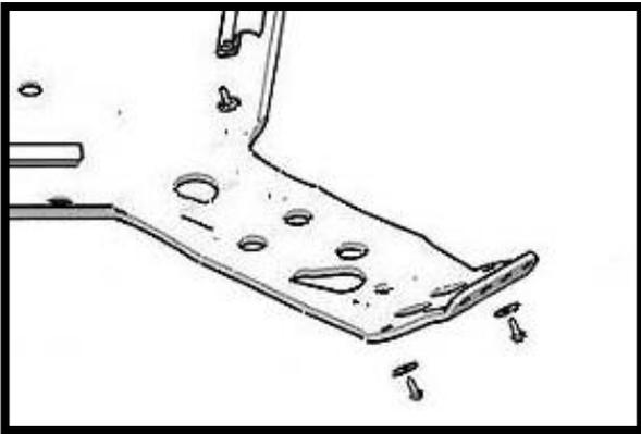
8. You can now use your factory washers from step # 6 and move them to the back side of the bumper guard. Then re-install it using factory hardware and fasten all skid plate screws.
