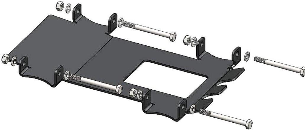
6. **If you have a rock crawler edition**, you can now LOOSELY reattach the skid plate back to the frame. This will help when securing it at the front in the next couple steps.
