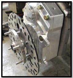
b. Slide on the supplied **30mm lock washer**, followed by the **30mm spindle castle nut**. (46mm) [**Min 120 ft lbs**] Tighten the castle nut further if needed to align grooves with holes in the spindle for the cotter pin. Install the supplied **cotter pin**. Both ends of the cotter pin must be folded.
