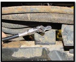
g. Route the new **96" rear left** (driver side) and **96" rear right** (pass. side) brake lines from the t-block and back down to the calipers. Make sure the orientation is correct and secure the new brake lines to the t-block. And then attach the brake line to the caliper.
