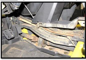
b. Disconnect the factory t-fitting from its fitted section. And then remove the nuts securing the factory brake lines to the bottom of the seat frames.
