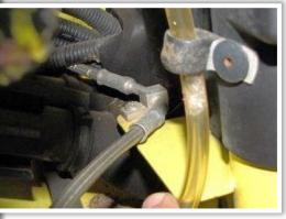
d. Disconnect the front supply line from the master cylinder under the steering wheel. **Have area prepared for brake fluid clean up**.
