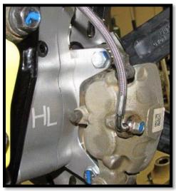
h. Next, pull any extra slack out from the caliper to under the seat. Then re-use your **factory p-clamps** to secure the new brake lines to the trailing arms. Insert a **6mm x 12mm screw** through each clamp and fasten them. **Do not over-torque!**
