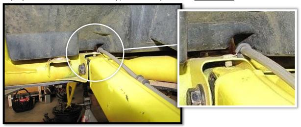
e. Disconnect and remove all <u>rear</u> brake lines from the master cylinder. Start by disconnecting the rear supply line from the master cylinder under the steering wheel. **Have area prepared for brake fluid clean up**.
