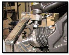
c. Position the lower ball joint into the lower ball joint mounting bracket on the backing plate.
