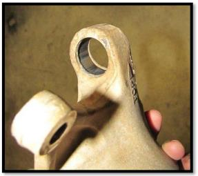
d. Inspect the radial joints for excessive wear or damage. If they show significant signs, they need to be replaced.
