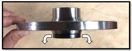
c. With the shorter lip side faced down, find the bolt pattern that corresponds to your make and model. Use the provided studs PGLC-WSTUD-102 (12mm-1.5 stud) (4/137mm bolt pattern)
