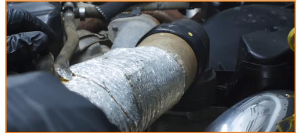
4. Lubricate the inside of the connectors on the Mishimoto upper radiator hose.
