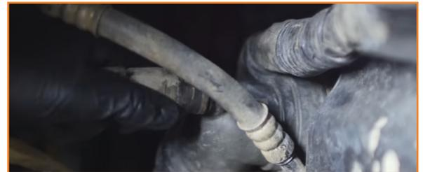
7. Pull the clip that holds the lower radiator hose on the radiator. Then slide the lower radiator hose off the connection.
