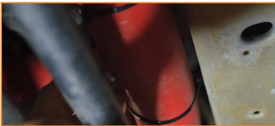
15. Fill the cooling system with premixed, Ford-approved coolant, start the engine, and allow it to idle with the cap off. Turn the heater control valve on the vehicle's HVAC unit to full hot, and put the fan on low. Monitor the engine
