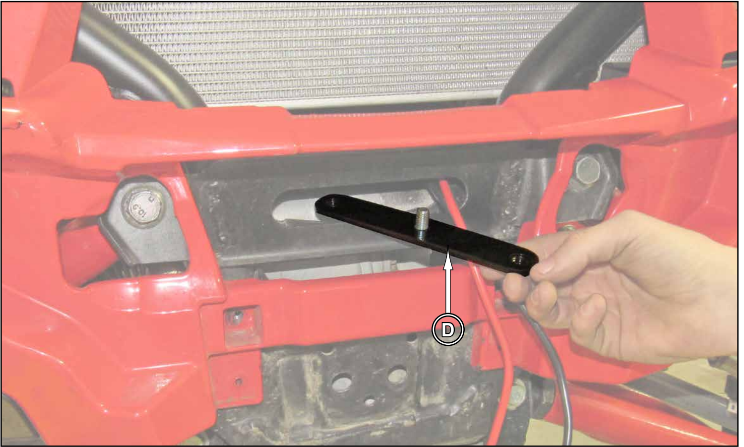
- Install Backing Plate (D) to Frame with hardware shown.
