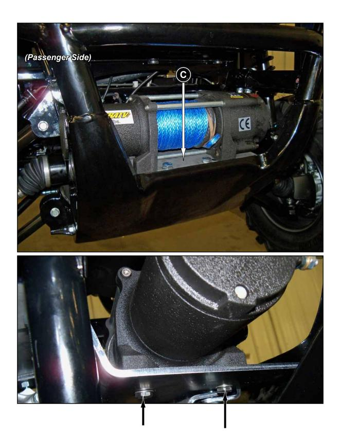
Secure to Mounting Plate (C) using hardware included with Winch
