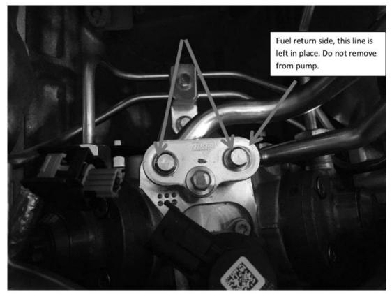
Remove the "T-bar" shown in the picture above stamped "FoMoCo" by loosening the 10mm flanged head bolt. This bolt will be reused to attach the failsafe adapter.
