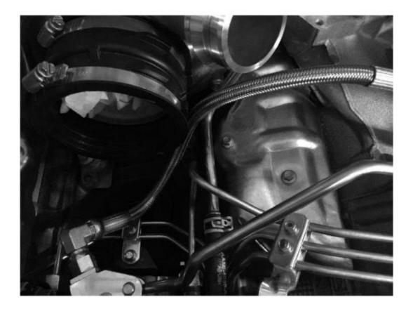
The line bracket that holds the supply and return hard lines is modified to allow attachment of the new 2 wire braided hydraulic line by removing one of the "Christmas tree" posts closest to the bracket mounting hole allowing the plastic snap to rotate and clear the 2 wire braided hydraulic crimp collar. Top is modified and bottom is unmodified. This is required for both versions of the kit.
