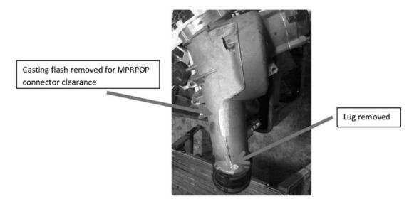
The casting flash rib in the area shown above should be removed to avoid interference with the MProp connector when the manifold is reinstalled.
