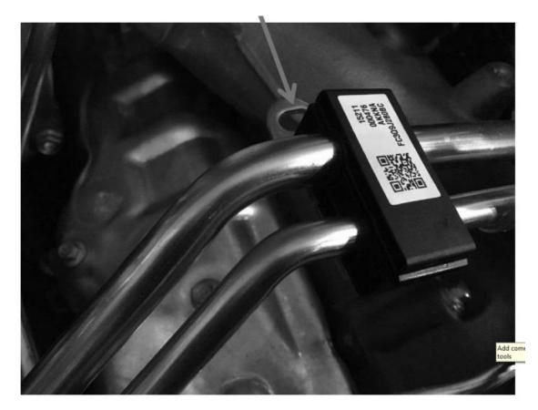
**\*\*NOTE\*\*:** Before proceeding, carefully clean the top of the high pressure pump and surrounding areas to remove any loose dirt or debris as it is critical no contamination finds its way into the fuel system. This step can be dismissed at your own risk. When working with fuel systems, cleanliness is an absolute must. After cleaning, remove the circlips on both the supply (left side) and return (right side) fitting as shown.
