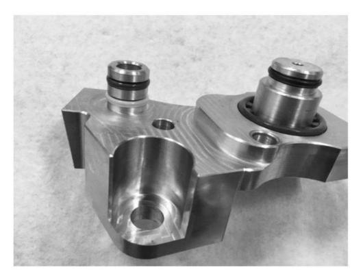
Install adapter block into pump after lubing o-rings. Use caution to avoid cutting o-rings on install.
