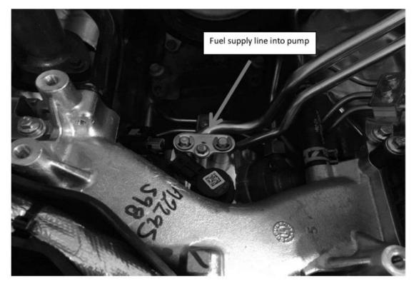
Removal of the fuel filter and fuel filter base housing is required to gain clearance to remove the upper plastic air manifold. Remove the hard plastic line from the filter to the fuel supply steel line that goes to the high pressure pump. The supply line to the pump is on the passenger side of the pump. See pic above. Then the aluminum manifold can be removed. The lug on the bottom of the aluminum manifold should be cut/ground off as shown to ease later reinstallation.
