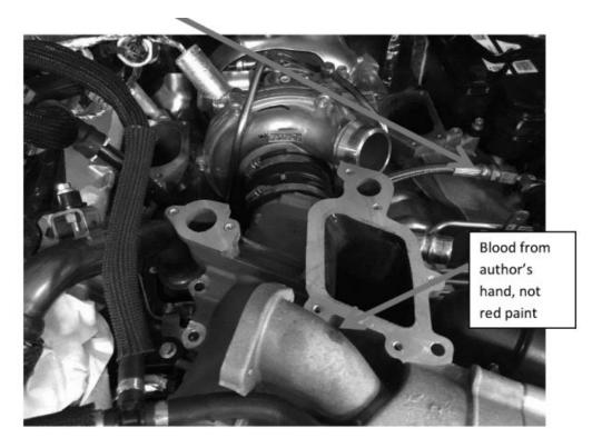
The modified hold down bracket above can now be reinstalled and the new fuel supply line and return line fit, tightened and clamped in place, making sure the 2 wire braided hydraulic supply line does not touch any components. On the models with a single sensor on the supply line, the 2 wire braided hydraulic line can be clamped in the modified stock plastic hold down block. The block can be swiveled allowing closure of the snap block around the 2 wire braided hydraulic part of the feed line.
