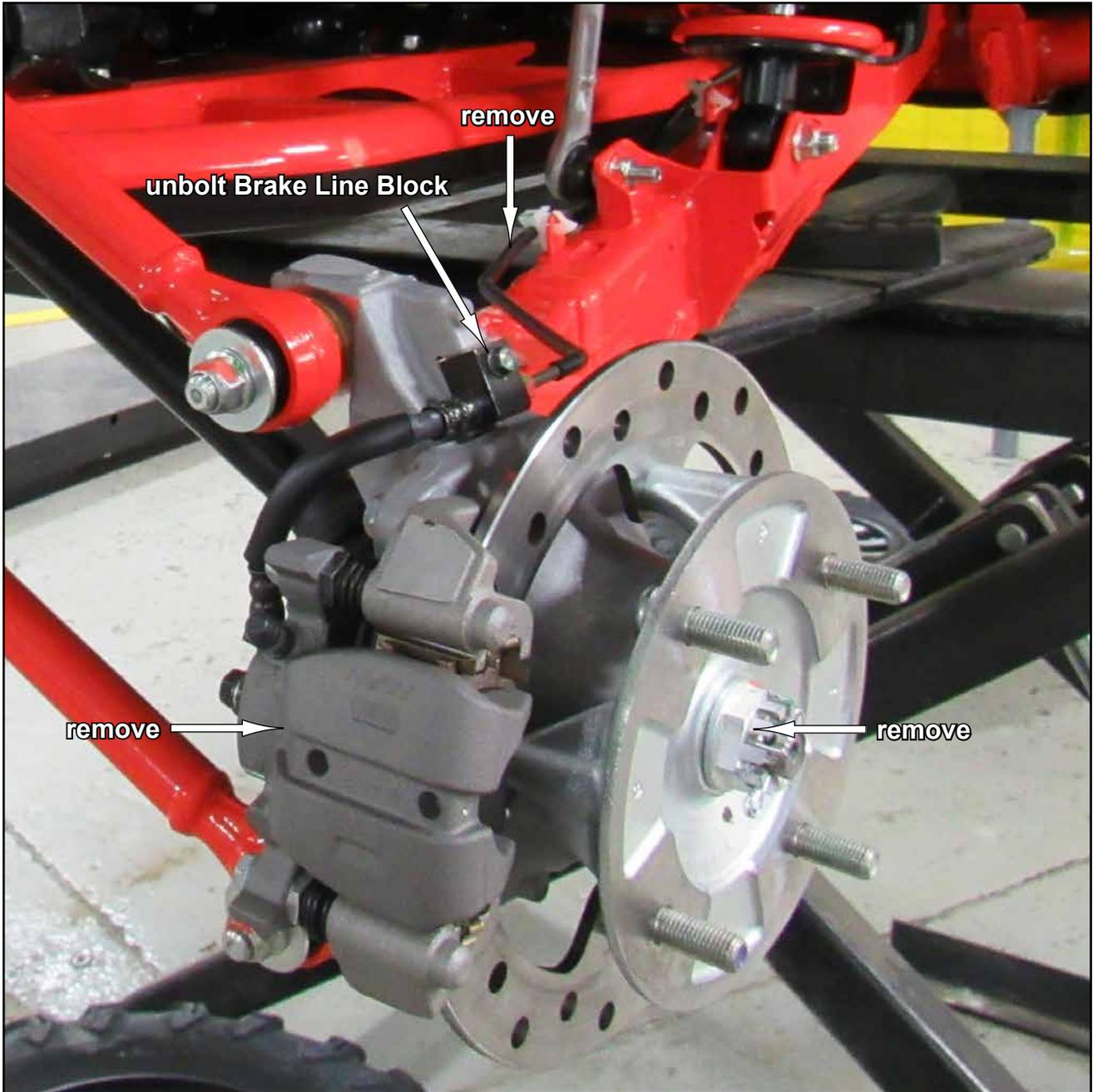
**Rear Components Removal continued:** *Keep all components removed from machine.*
