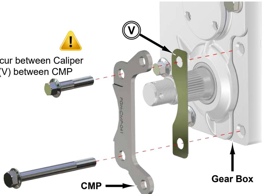
**Rear:** do not tighten hardware completely unless noted.
