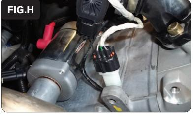
Plug the mating pair of 3-pin connectors on the PCV wiring harness in-line of the TPS and the stock wiring harness (Fig. H).
