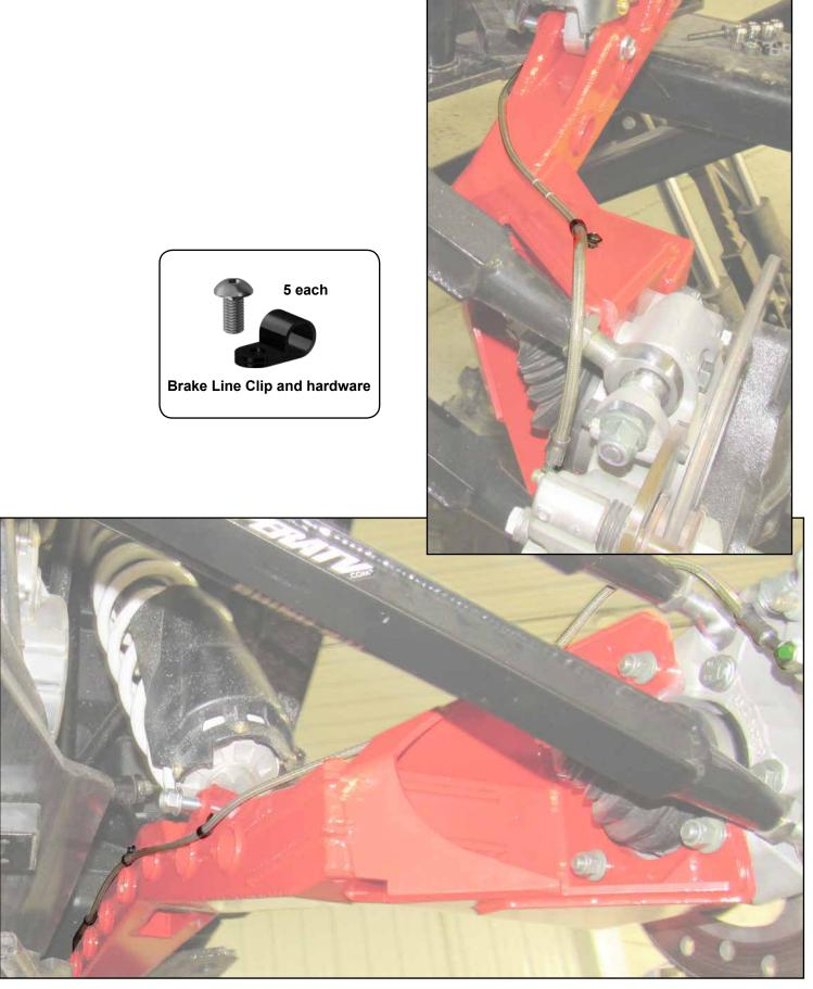
Tighten all hardware completely and repeat steps for driver side.
