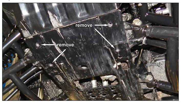
do not tighten any hardware completely unless noted
