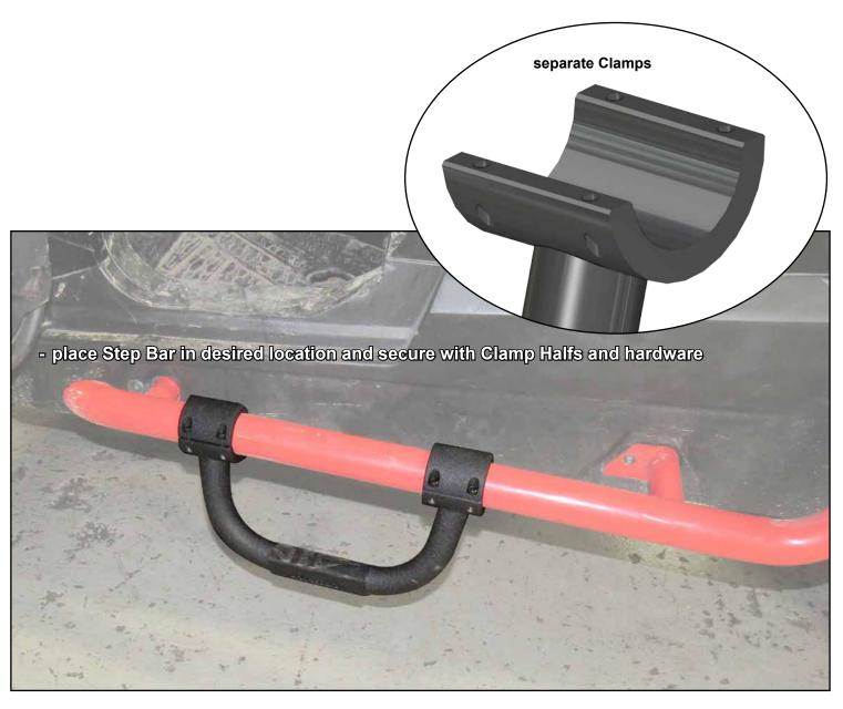
tighten hardware completely and repeat steps for opposite side
