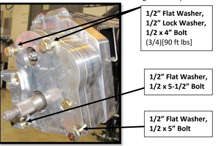
d. Slide a ½" flat washer onto each bolt end and fasten each with a ½" lock nut. (3/4)[105 ft lbs]
