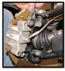
b. Remove the front brake scraper from the caliper, it is no longer needed. (8mm)
