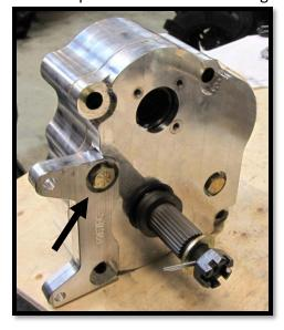
c. Insert the washers and bolts below through the remaining four holes in the front of portal box.
