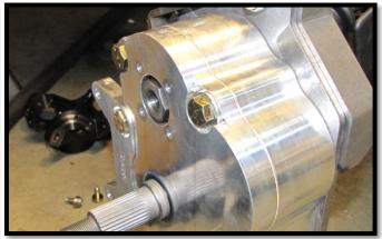
c. Align the portal box lid cap & gasket. Use the (4) 8-32x1/2" screws and install to the portal box. [8 ft lbs]
