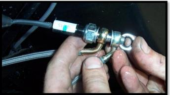
c. Install the new longer brake line **PGLC-BRAKELINE** to the banjo bolt. Run the line back through the frame and to the (PA) side hub.
