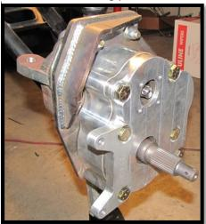
d. Loosely fasten the bolts with **½" flat washers** and **½" lock nuts**. Recheck all parts that were used and make sure everything fits correctly, and then go ahead and tighten and torque all 4 ½" bolts. (3/4)[105 ft lbs]
