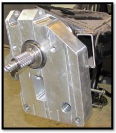
b. Install and fasten the backing plate to the trailing arm using (4) M10-1.25x35 bolts, (4) 10mm lock washers, and (4) 10mm washers. (15mm) [50 ft lbs]
