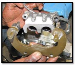
b. Find the new rear brake caliper hanger bracket **PGLC-BCB-85X.** Apply **LOCTITE (BLUE)** to the pins and fasten them to the bracket. [73 ft lbs] Then insert it into the brake caliper.
