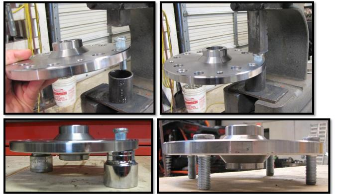
e. Once the studs are pressed in, locate and place (4) ½" brake rotor spacers (PGLC-ROTOR-SP) over the tapped holes.
