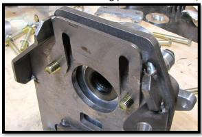
f. Reconnect the upper ball joint mount bracket to the portal box. Check the camber again. If it's correct, proceed to step #7. If not, repeat the previous step until you achieve the correct angle.
