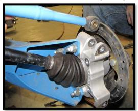
d. Remove the cotter pin and loosen the rear wheel hub castle nut (27mm). Remove the nut from the rear wheel hub assembly. Then remove the brake rotor assembly.
