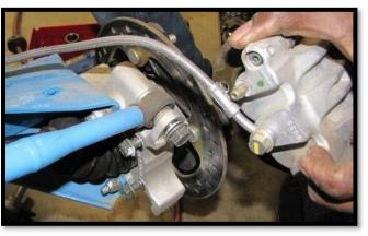
c. Remove the bolts and nuts that attach the rear knuckle to the radius bars. (15mm)
