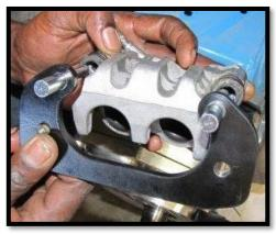
c. Install the caliper onto the portal box between the new caliper bracket and rotor. Use the supplied M10X1.25X25 bolts and 10mm washers (These are replacing the factory 50mm bolts). (15mm) [30 ft lbs] Position brake line banjo fitting clocked to 10 o'clock so it runs at the proper angle for maximum suspension travel. Tighten & torque to specifications. (13mm) [15 ft lbs]
