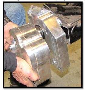
c. Insert the washers and bolts below through the rear portal box. Fasten the top two bolts.
