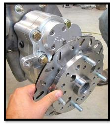
c. Slide on the supplied **30mm lock washer**, followed by the **30mm spindle castle nut**. (46mm) [**Min 120 ft lbs**] Tighten the castle nut further if needed to align grooves with holes in the spindle for the cotter pin. Install the supplied **cotter pin**. Both ends of the cotter pin must be folded.
