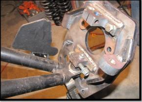
g. Insert the axle into the backing plate.
