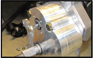
c. Align the portal box lid cap & gasket. Use the (4) 8-32x1/2" screws and install to the portal box. [8 ft lbs]
