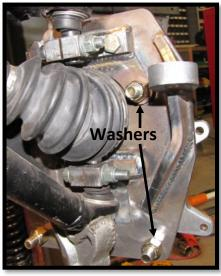
e. Install the tie rod end in through the top of the portal box tie rod mount bracket. Fasten the tie rod end with the factory nut. (18mm)[90 ft lbs]
