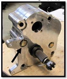
b. Apply grease to the axle drive splines. Make sure to apply product all around the outer edge as well. Rotate the portal box assembly "Up & In" as you guide the drive shaft axle through the inner drive gear.
