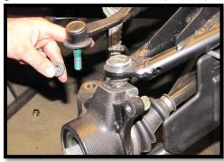
h. Remove upper ball joint pinch bolt from the knuckle (15mm). Then remove the lower ball joint nut from the knuckle. (18mm)
