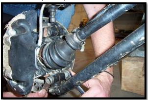
i. Remove the knuckle and retain the factory bolts & nuts. They will be re-used later in the install process.
