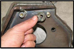
e. Properly position and insert the lower ball joint into the lower ball joint mounting bracket on the backing plate assembly.
