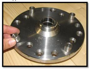
f. Locate a brake rotor **PGLC-ROTOR**. The side with the counter bores should be facing up. Place the rotor on to the hub and line the holes up with the tapped holes.
