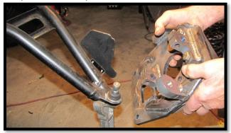
f. Secure with the factory bolt and nut. (18mm)[90 ft lbs]
