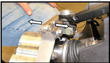
e. Now that the backing plate is accessible, remove or add shims as needed.
