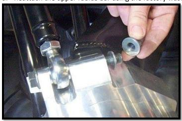
b. Reattach the lower radius bar using the factory washer and lock nut. (18mm)[90 ft lbs]
