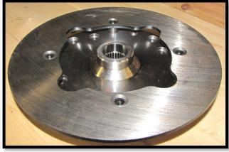
g. Apply **LOCTITE (RED)** to (4) **3/8-16 x 1" button head bolts (BSH381)**. Insert the screws through the rotor, the spacers, and then into the hub. Tighten and torque. [45 ft lbs]
