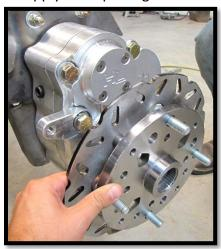
a. Slide on the supplied **30mm lock washer**, followed by the **30mm spindle castle nut**. (46mm) [**Min 120 ft lbs**] Tighten the castle nut further if needed to align grooves with holes in the spindle for the cotter pin. Install the supplied **cotter pin**. Both ends of the cotter pin must be folded.
