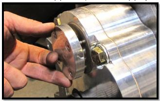
b. Using the pre-installed ½ x 2 1/4" bolt, 1/2" lock washer, and 1/2" flat washer. Insert it through the upper hole of the caliper mounting bracket PGLC-BCB-81G and place it in the corresponding fitted section of the front portal box and fasten it tight. (3/4) [90 ft lbs]
