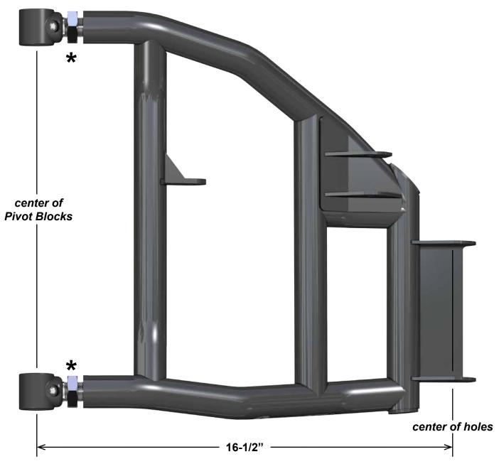
\*Leave Jam Nuts loose. Tighten after final adjustments have been made.
