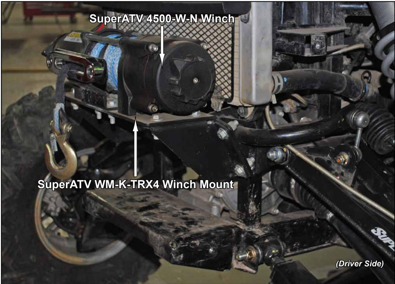
**!** Remove Insert from Lower (D) if a Winch is installed in position shown above.
