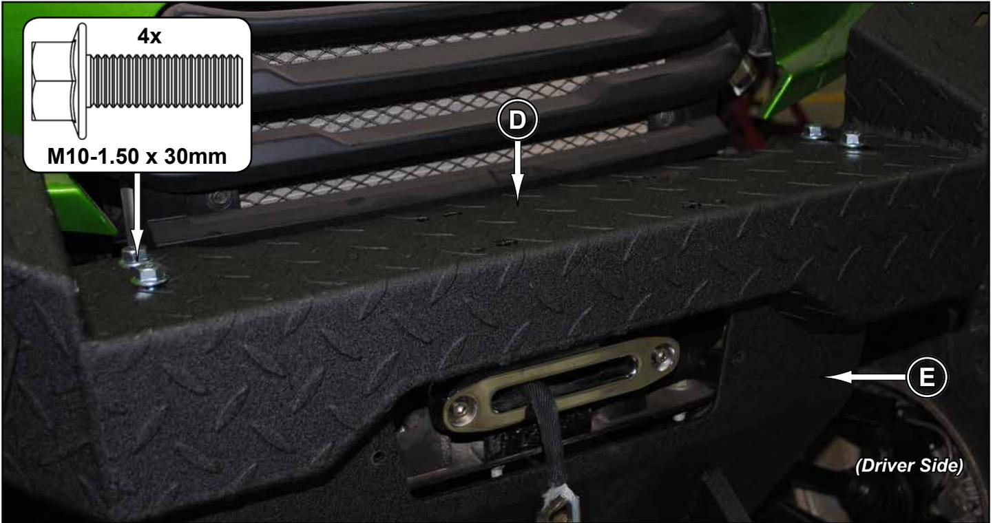
*Align to machine and tighten all hardware completely.*
