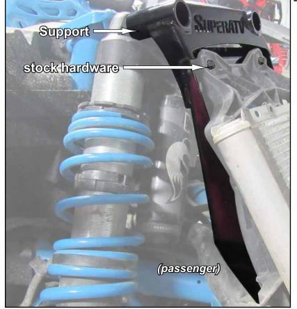
Remove spacer and secure Shocks and Radiator with stock hardware.
