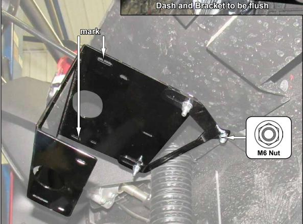
Remove Bracket and drill holes, large enough for Ø6mm bolts, into Dash. Leave Bolt in place.
