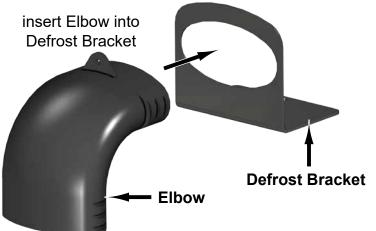
secure Defrost Bracket with hardware shown
