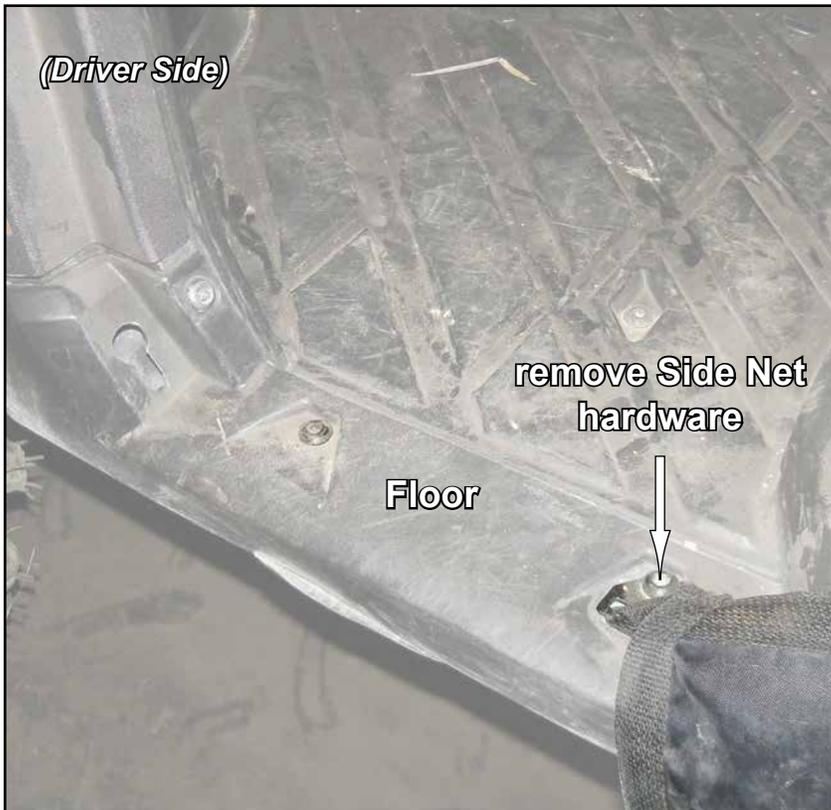
*Do not tighten hardware completely unless noted.*
