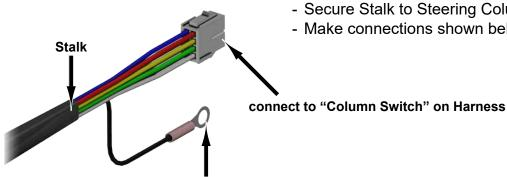
ground to Steering Column with stock hardware shown
