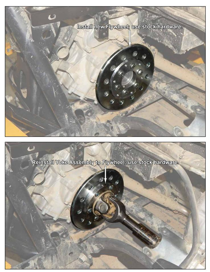
Reinstall previously removed stock components.
