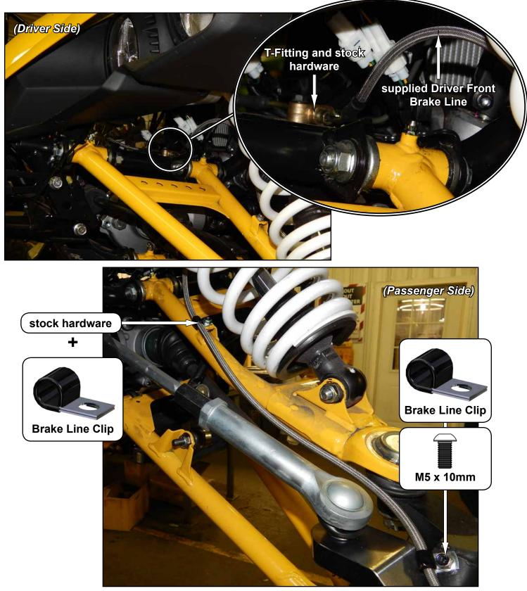
**Rear:** do not tighten hardware completely unless noted.
