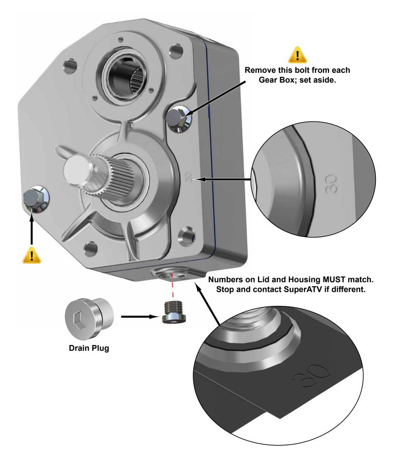
Remove Components from each side: Keep all components removed from machine.
