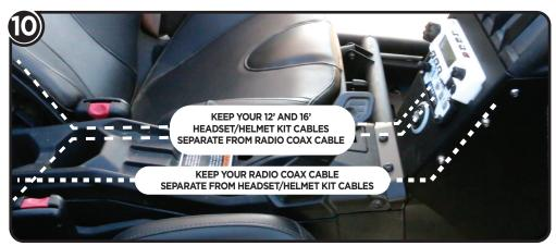
Begin the process of running your cables through the vehicle. This includes your power cables, antenna coax cable, and 12' cables for front seat and 16' for rear seats. Pay attention to where you're plugging in your PTT (Push-to-Talk) buttons. Be sure your coil cord driver-side PTT button is plugged into the Driver PTT port and the co-driver straight-cord
