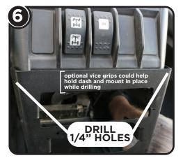
With the bracket placed in position, secure the bottom 2 Torx screws that you removed in the previous step. Position the dash/top of the mount to the same bottom line of the rocker switch separators that we used for the sticker. Vice grips may be a good option to hold the dash and the mount in place. Once lined up, drill holes in the left and right side using a 1/4" drill bit. Do not attach the top bolts to secure the mount just yet. Now remove the bottom 2 torx screws to remove the bracket.
