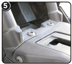
Next, remove the bottom 2 torx T-30 bolts in between the console pillars.
