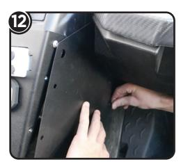
Follow the next step if you are installing the optional side panels. On the passenger side, start by removing two plastic rivets towards the back, closest to the floorboard. Next, place the side panel in place and insert the plastic rivets back into their holes. The panel can be lined up for the front bolts and secured. On the driver side, attach the 2 side bolts and secure.
