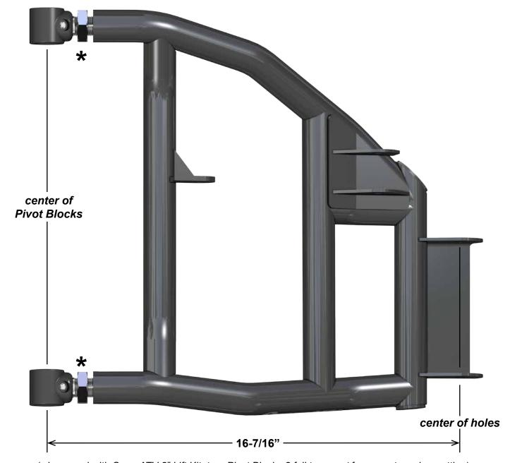
(when used with SuperATV 2" Lift Kit, turn Pivot Blocks 2 full turns out for correct camber setting)
