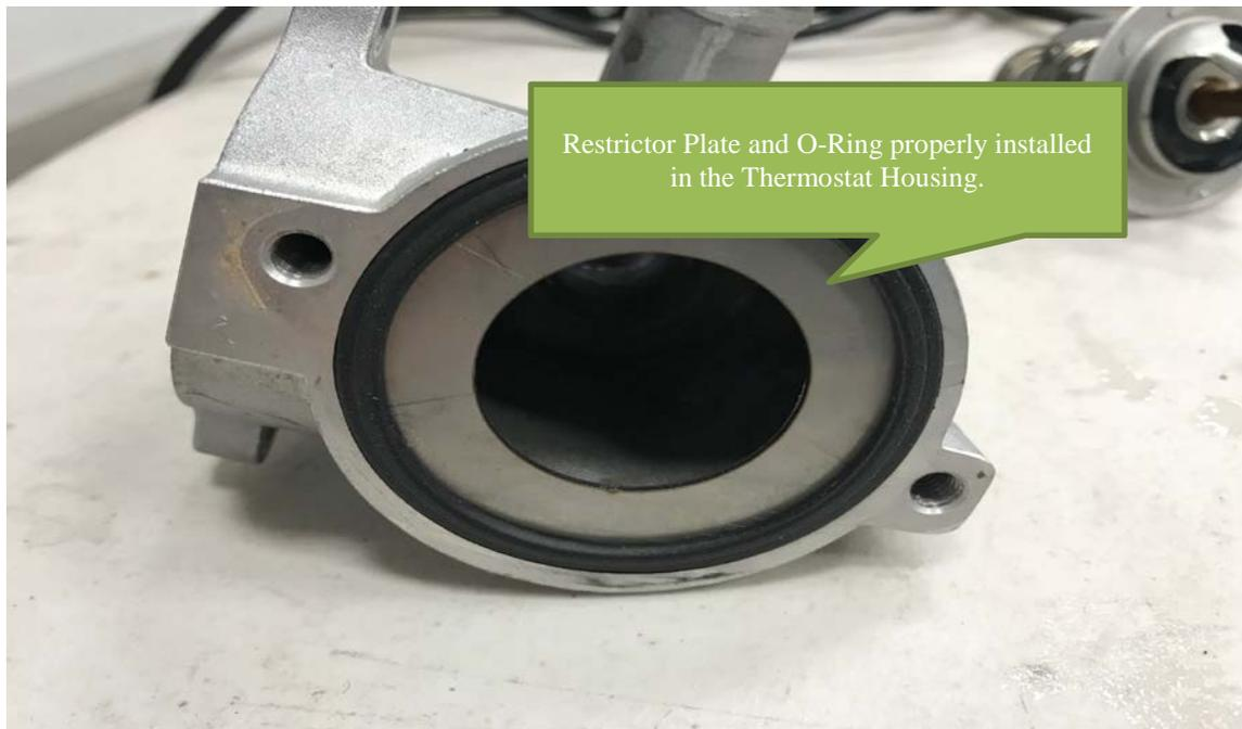
Step 6: In reverse of the previous steps, reinstall thermostat housing to engine, reconnect hoses and reinstall the muffler and any heat shields that were removed in previous steps. Leave upper T Stat housing clamp loose as you will burp the system here for air in Step 11. **PRO TIP: Align hose clamps to make access easier, some of the clamps are facing incorrectly from the factory and difficult to remove.**
