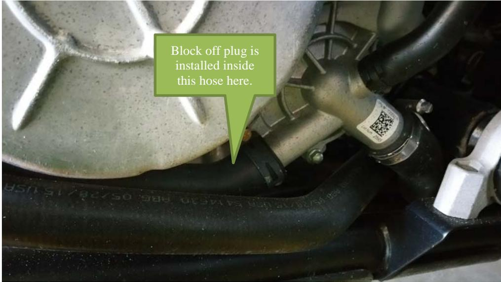
Step 2: Install supplied billet block off plug into the 7/8" coolant bypass hose as shown in the picture below. This is the same hose that was removed in Step 1.
