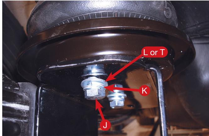
Align the holes in the lower bracket and roll plate to the threaded insert in the air spring and attach with (L or T), (K) and (J).
