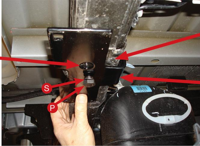
The frame has a ridge; the bracket must be parallel to this ridge.
