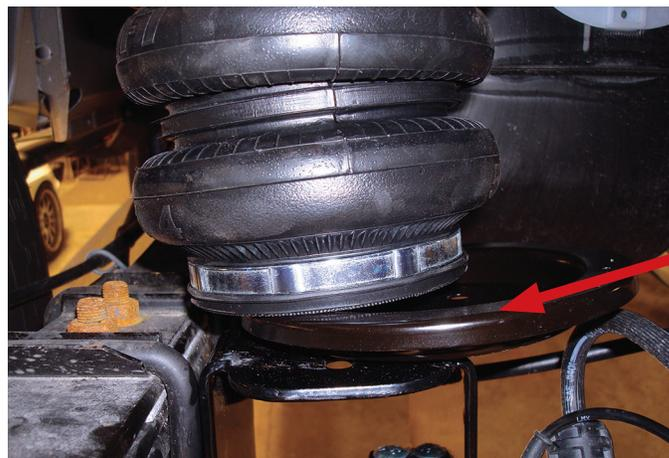
Slide the roll plate between the lower bracket and air spring while aligning the holes in all three.
