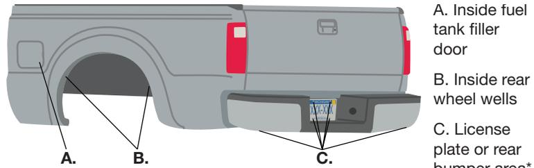
\* For LoadLifter 5000 Ultimate Plus kits, the recommended location for the Schrader valves is the rear bumper area or license plate.
