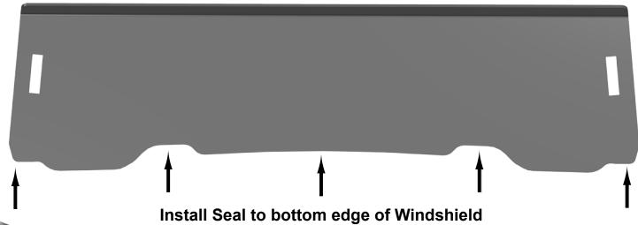
To ease installation, soak Seal in hot water before cutting or installing to increase flexibility.
