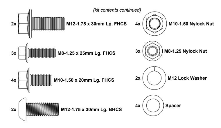
When assembling do not tighten hardware completely unless noted.
