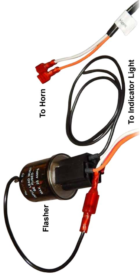
**Always consult Wiring Harness Diagram when making connections.**
