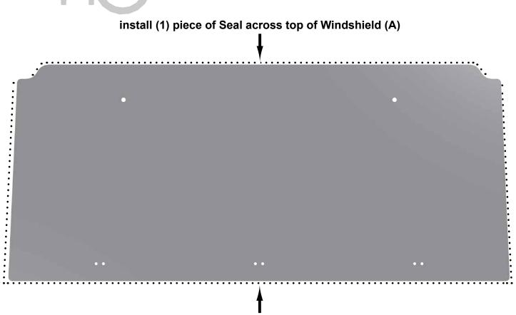
install (1) piece of Seal to sides and bottom of Windshield (A)
