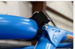
13. Install the Adapter (K) on the mounting bosses of the Particle Separator (F) with the supplied Screw (D) and Washer (E). Tighten these screws using a 4mm Hex Key. Install the spacers provided if installed on the top utmost bar on the cage. Note: Mounting on the top bar will require the use of the supplied Spacers (W), Screws (X), and Washer (E).
