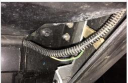
37. Use the supplied Posi-Tap (U) and unscrew the large top cap. Place the cap in between the orange/green wire.
