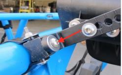
17. Go over all the screws and locknuts again to make sure they are secure and that the Particle Separator (F) is firmly attached to the roll cage.
