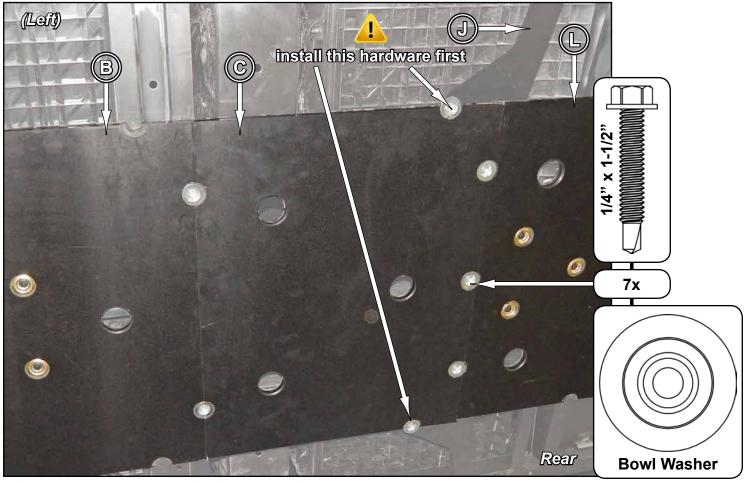
Slide Left Rear Guard (H) under Rear Plate (D) and secure to Frame with hardware shown.
