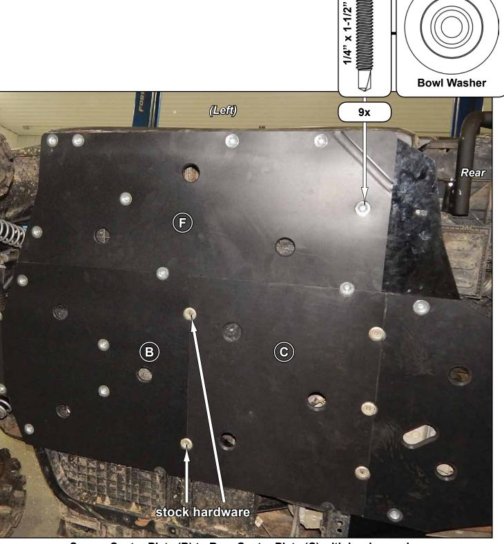
Secure Center Plate (B) to Rear Center Plate (C) with hardware shown.
