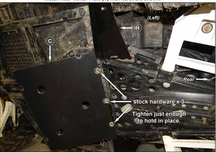
Install Rear Plate (D) to Rear Center Plate (C) and Left/Right Guards (H)(G) with hardware shown.
