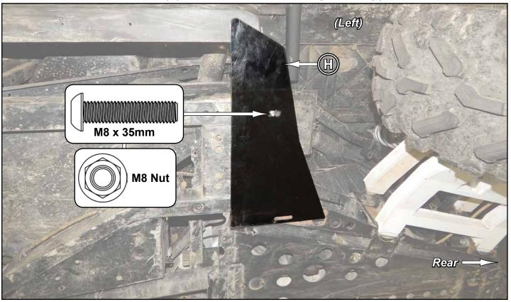
Install Rear Center Plate (C) with hardware shown.
