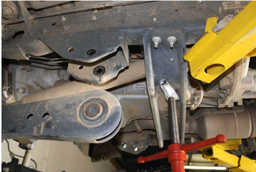
Figure 13: support the cross member, then remove the nuts.
