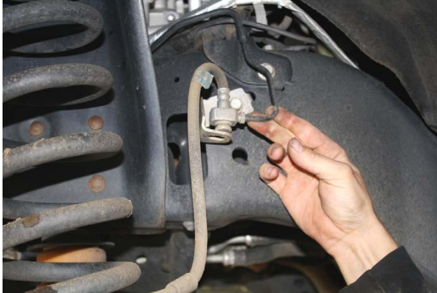
Figure 5: brake line removed from frame bracket
