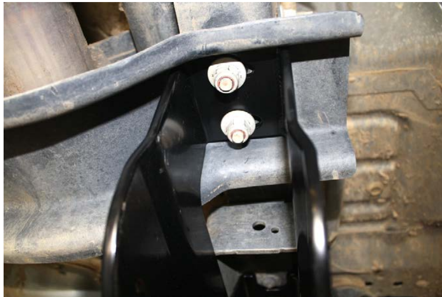
Figure 12: install the factory nuts to hold the rear of the radius arm bracket in place.
