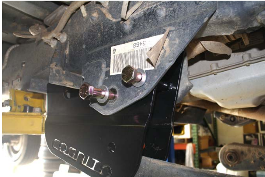
Figure 11: install radius arm bracket, with supplied hardware
