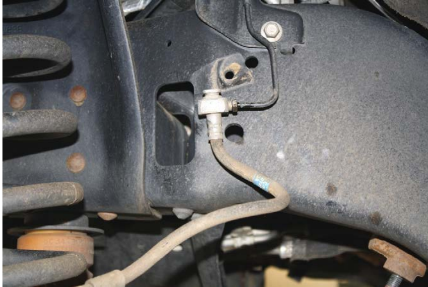
Figure 7: brake line rotated, fitting retightened.
