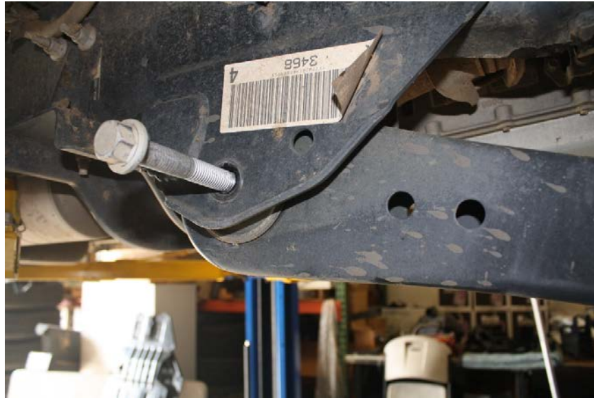
Figure 9: unbolt radius arm from frame
