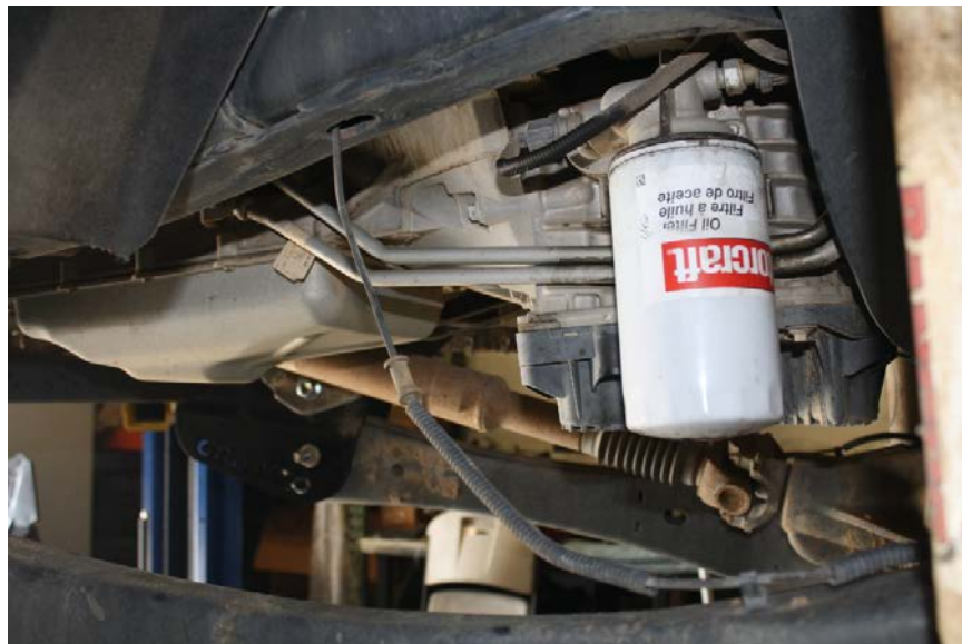
Figure 16: re-route the ABS sensor cables
