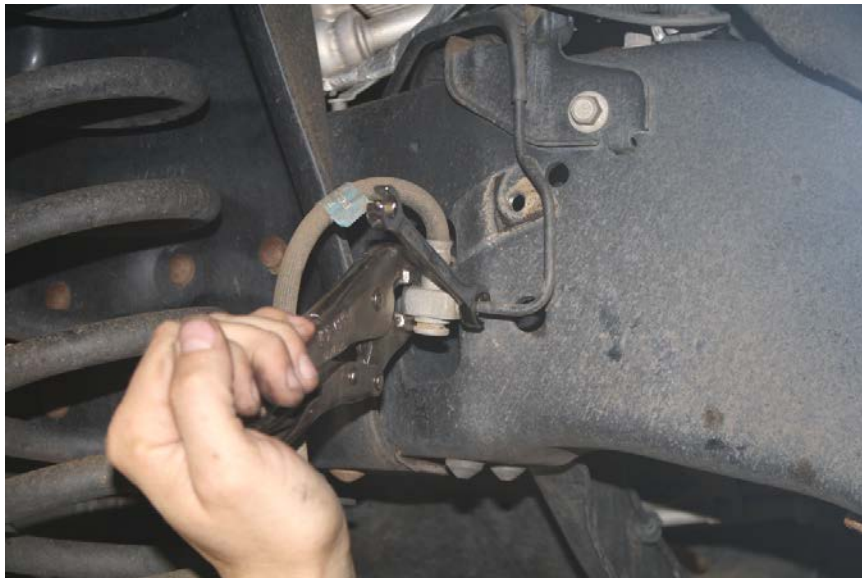
Figure 6 brake line preparing for rotation
