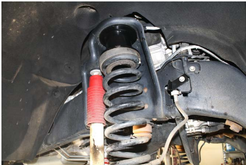
Figure 14: install the coil spacer and coil spring as an assembly, into the stock location.
