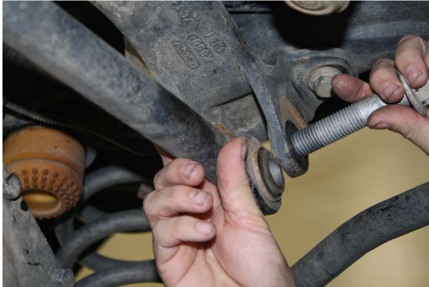
Figure 1: remove torsion bar adjusting bolt
