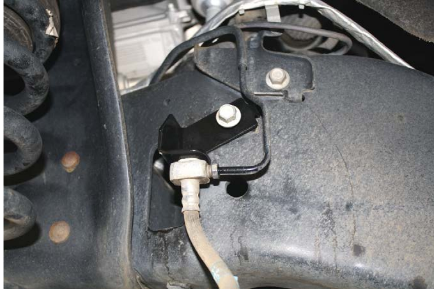
Figure 15: fasten the brake line to the new bracket.
