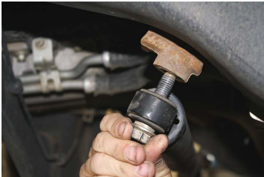
Figure 2: unbolt only passenger side of the steering stabilizer
