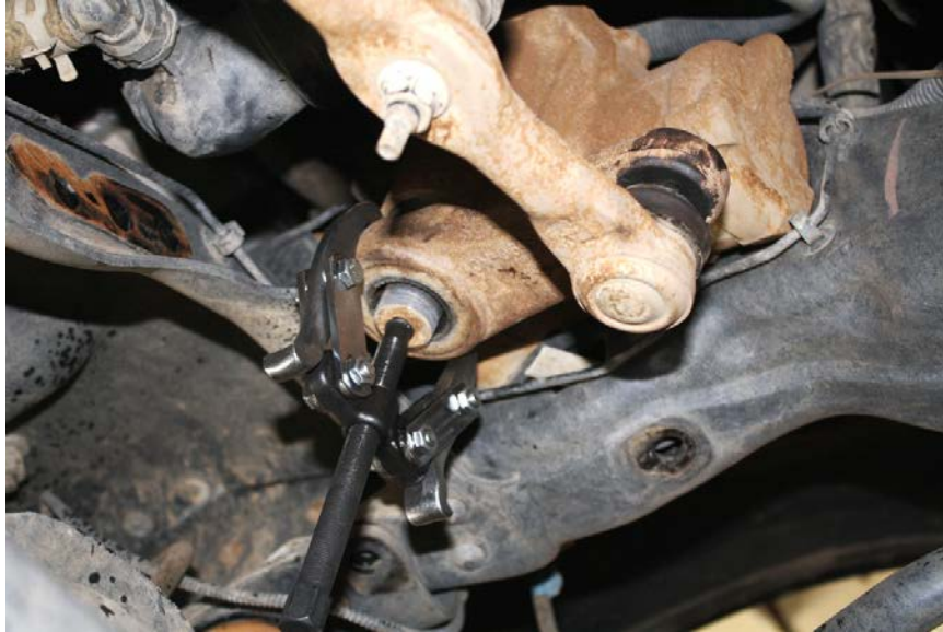
Figure 3: remove pitman arm from steering box
