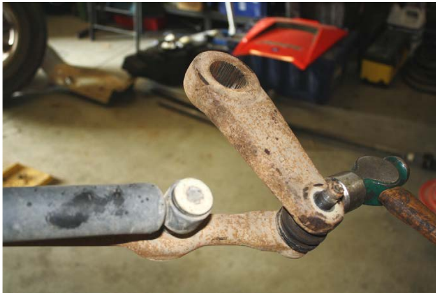
Figure 4: remove pitman arm from drag link
