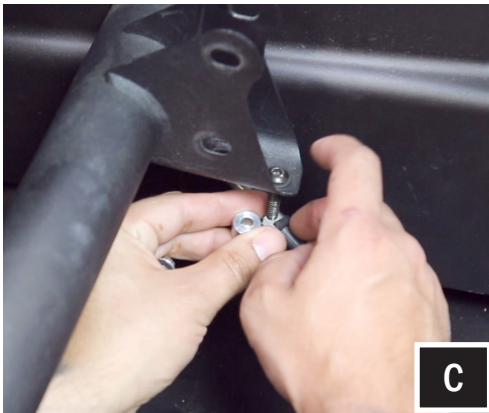
C. Remove the factory 10mm nut and bolt from the brake line. Place the washer on top of the factory bracket and push the long M6x25mm screw through the top. Then attach the brake line, spacer, washer and nut. Then hand tighten.
