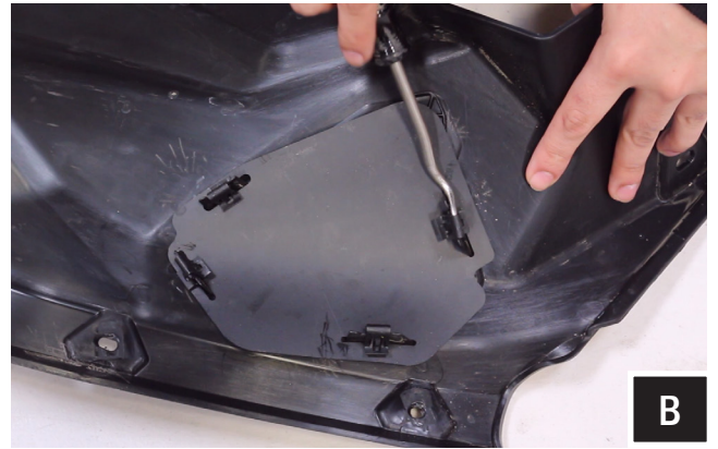
B. Pry off the (4) clips on the base under the empty space for the speaker
