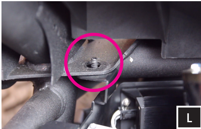
L. Make sure the threaded bolt on the amp plate goes through the factory hole located in the corner where the cage tubing connects.
