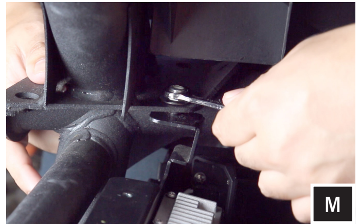
M. Secure the amp tray to the vehicle using the supplied M6 nut and washer.
