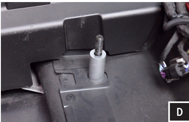
D. Replace the factory seat bolt spacers with the supplied SSV Works spacers
