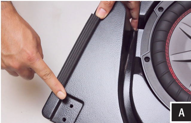
A. Apply the foam strips to the inside right, left and top side of the enclosure.
