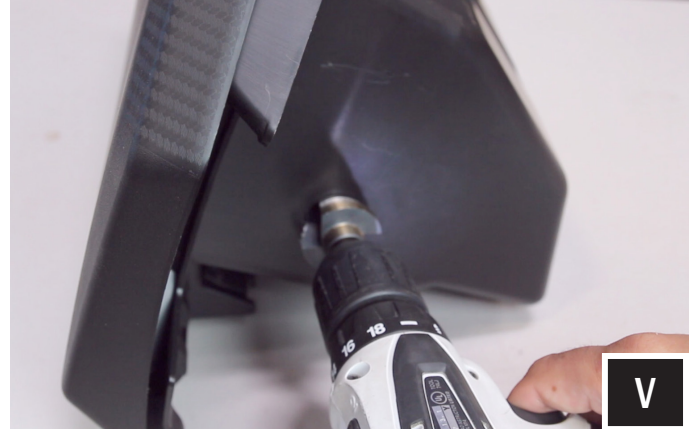
V. Drill a 1" hole through the left side of the glove box for wiring
