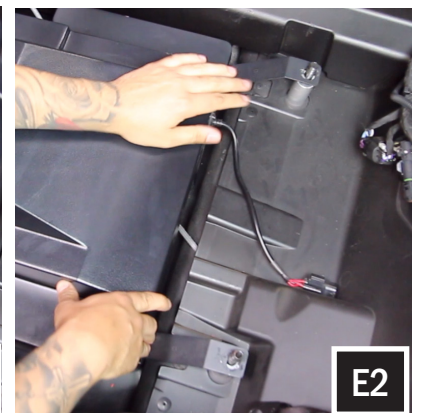
E. Run the brake line along the dedicated channel on the sub enclosure while feeding the enclosure down under the seat bar (F1). Make any adjustments to the brake line so the enclosure lays on top of it. Line up the rear enclosure brackets to the rear seat bolts and press down until the brackets rest on top of the spacers.
