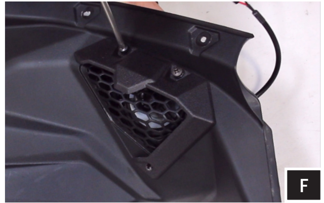
F. Place the speaker pod under the dash panel and line up the holes on the speaker pod with the (2) top screws and loosely mount the pod to the dash panel.
