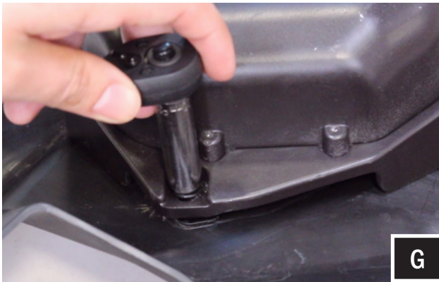
G. Insert the M6x25mm screw by pushing it through the acoustic lens, dash panel and speaker pod. Secure screw using washer and 10mm nut. Now fasten the previous (2) M6x1.0 screws.
