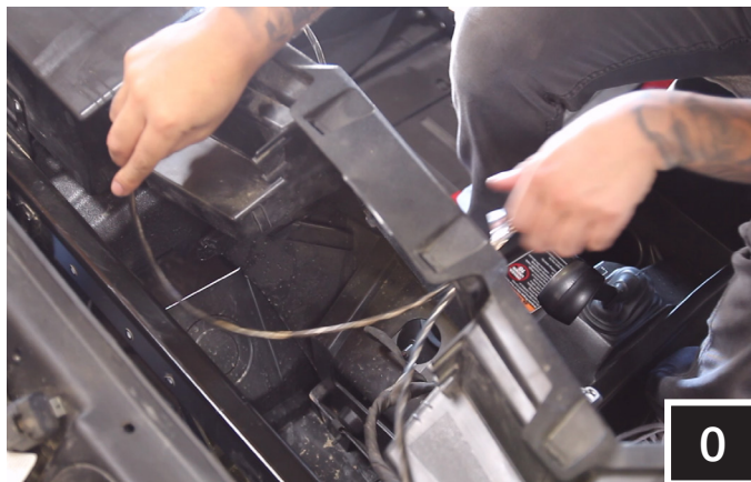
O. Route the H1149 harness towards the driver and passenger side of the dash.
