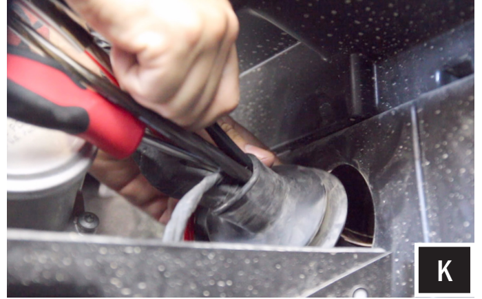
K. Unwrap the tape from rubber grommet and feed the power/ground wire for the Amp through the grommet as well as the rear speaker harness H1151 (rear speaker harness to be used for rear speaker expansion pods).
