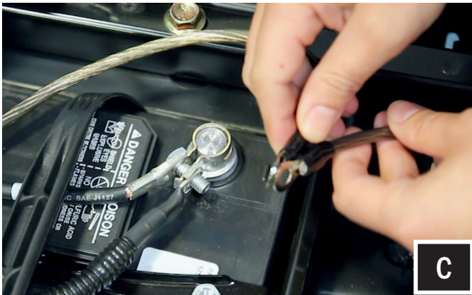
C. (If you have decided to disconnect the negative terminal as suggested earlier). Reconnect the negative battery cable. Remove the nut and connect the two ground cables. Reinstall nut and tighten.
