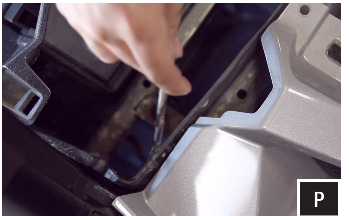
P. Feed each side of the H1149 harness down through the open cavity on top of the dash towards the driver and passenger footwell.
