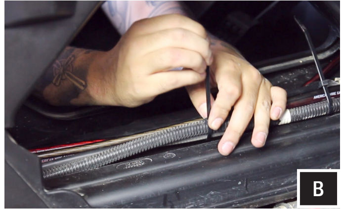
B. Zip tie all cables to the factory cabling along the center column away from the drive shaft.
