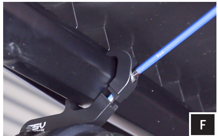
F. Using a T5 hex key tighten clamp until it secures to cage.
