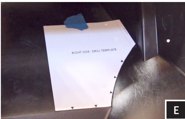
E. Cut out the RIGHT template along the cut line. Position the template on kick panel in the passenger footwell above the foot rest making sure to line up arrows on template to the curves of the panel as seen on image E.
