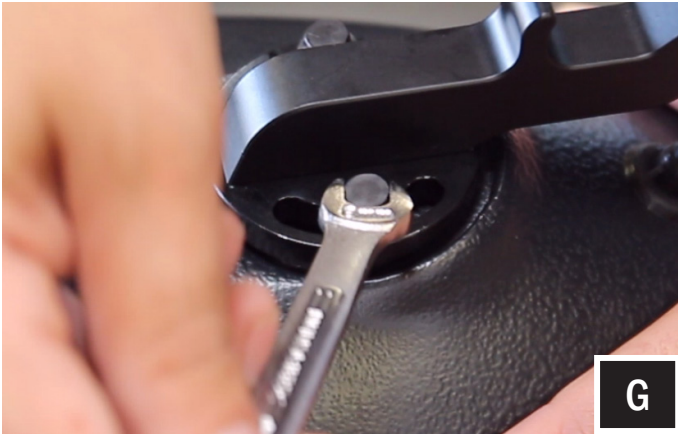
G. Tighten the 8mm bolts once you have the speaker pods in your desired location.
