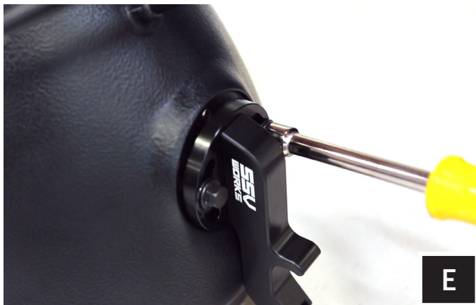
E. Loosely install the clamp base to the cage mount pod with the two (2) 8 mm head bolts and washers, place the cage mount pod in the desired mounting location on the vehicle.
