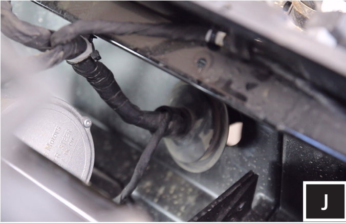
J. Unplug the rubber grommet located on the firewall.
