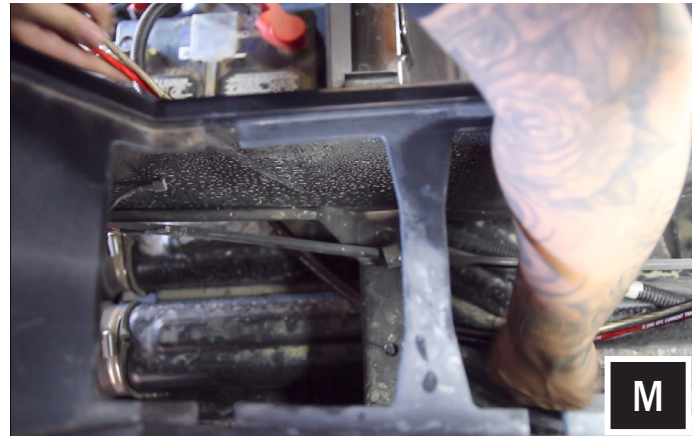
M. Follow the air ducts and factory wiring and feed cables towards the back. (use provided zip ties to secure cables to factory wiring, away from the drive shaft).
