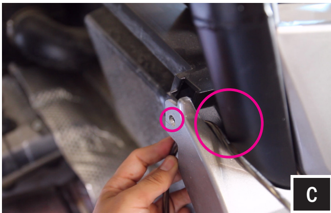
C. Remove push clip on the rear panel to allow the running of the speaker harness up the driver and passenger cage bar to connect to the speakers.
