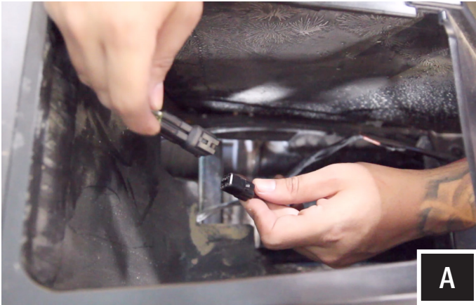
A. From the rear of the center console, connect the B-H1150 harness and route to the rear driver and passenger side from under the console.
