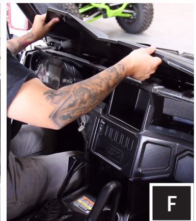
F. Use a panel removal tool to release the top of the dash. Lift up and completely remove the top of the dash panel.
