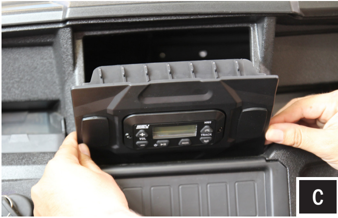
C. Place the bottom edge of the kit on dash.
