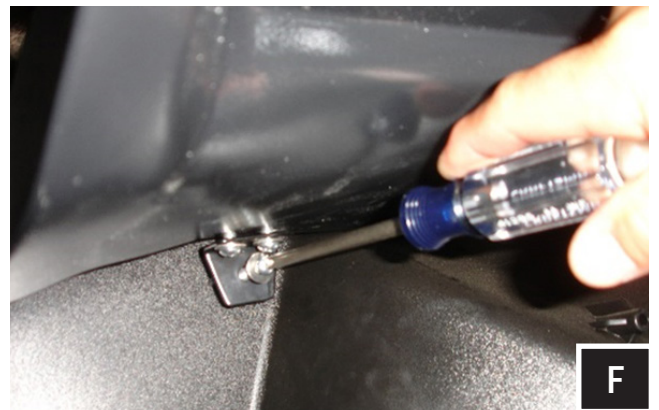
F. Loosely install the bottom L bracket, align the mounting hole with the factory bung and secure with one of the long screws provided (you will tighten the bracket to the enclosure and factory bung AFTER step J)
