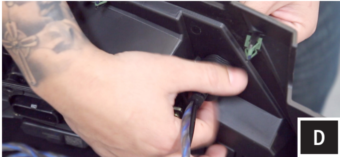
D. Feed the plastic nut back through the wires and cables and screw back onto the port. Hand tighten only. Replace fuse and close fuse holder.
