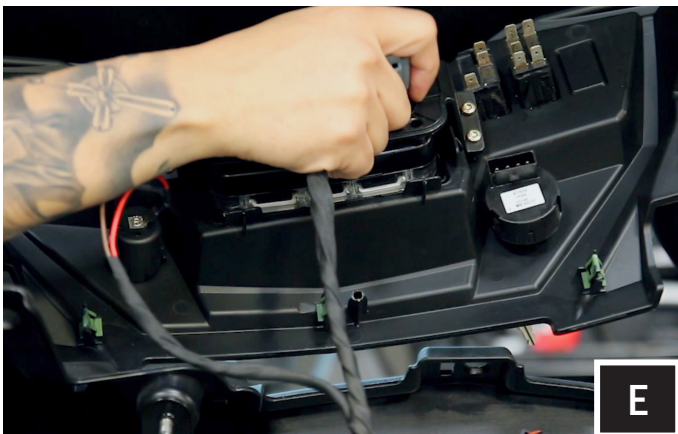
E. Disconnect all harness connectors attached to the center dash panel.
