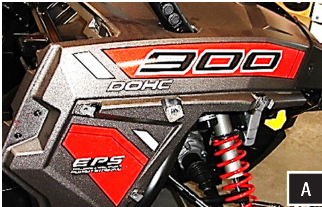
A. Remove the ten T40 Torx bolts that secure the 2 piece fender. Note: there is one screw inside the fender well. Remove the two additional screws from the striker plate, slide fender up the cage rail and secure
