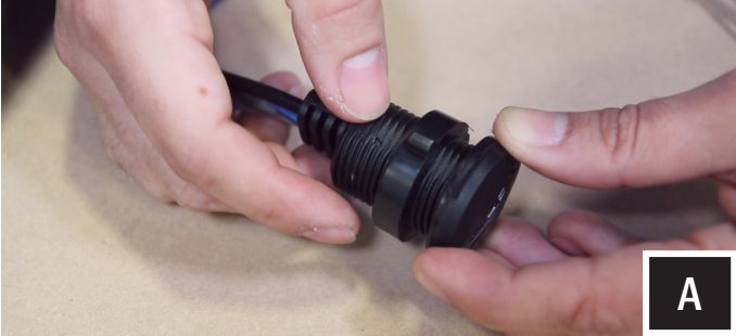
A. Unscrew and remove the plastic nut from the port. Make sure to open the fuse holder and remove the fuse so the nut will fit through it. Crimp on the provided ring terminals on the ends of the (Red) Power and (Black) Ground wire.
