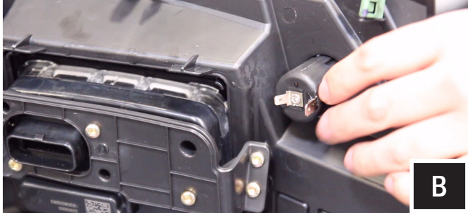
B. Make sure all harness connectors are unplugged from the dash panel. Push out the factory 12v port.
