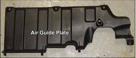
Air Guide Plate will not be reinstalled
