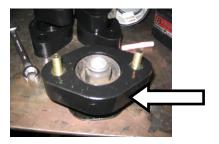
9. With the spacer mount installed. Install the mount into the fame support. **NOTICE: When** installing the front grill mount put the 2 studs in grill frame first, using the 2 studs and nut to hold the mount in the grill.
