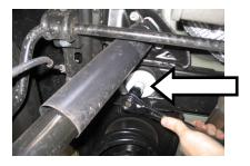
5. Place the floor jack under the Jeep tub between the front and rear wheel. Rise up the jack with the 2x4 jacking block on top of the jack and remove only one side at a time of the bolt and nuts from the Jeep mounts.
