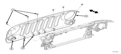
4. With a 16mm socket loosen the two nuts at each of the front core support body mounts, Then with a 18mm socket loosen the bolts at the right and left sides of frame body mounts. **NOTICE:** DO NOT remove nuts at this time. **NOTICE** a 2dr will have 10 mount and a 4 door will have 12 mount locations.
