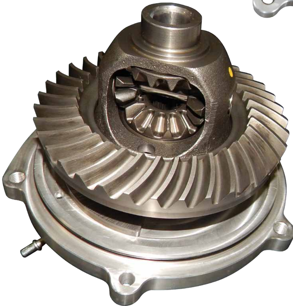
place Ring Gear Plate/OE Carrier Half assembly onto Lid
